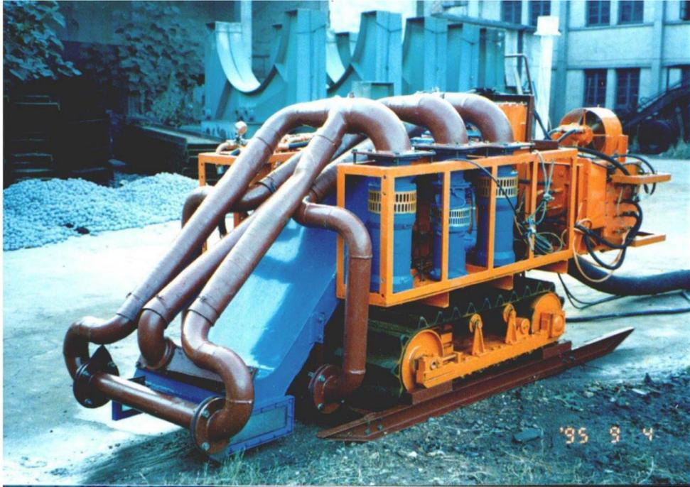
**Figure 1.4-2 Prototype of hydraulic collector vehicle**
