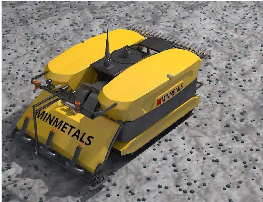
**Figure 1 Conceptual model of Minmetals collector vehicle**
