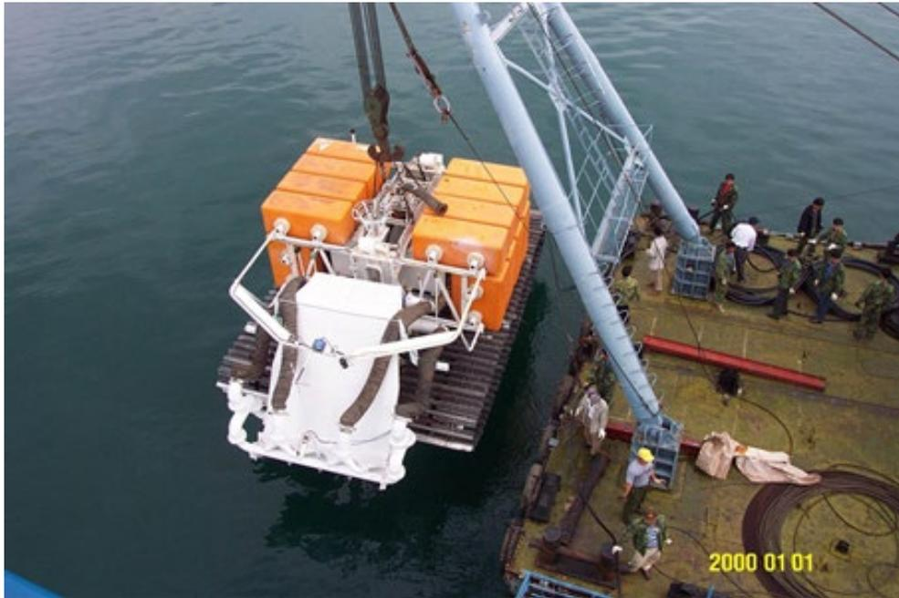
**Figure 1.4-3 Engineering PCV for lake test**
